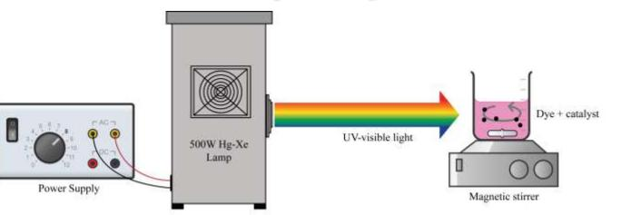
Schematic diagram of a photocatalytic reactor setup for the organic dye degradation experiments
