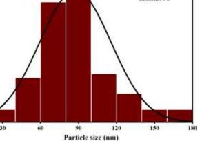
• FESEM imaging and particle size distribution revealed significantly improved morphology and reduced particle size due to Bi<sup>3+</sup> doping.
