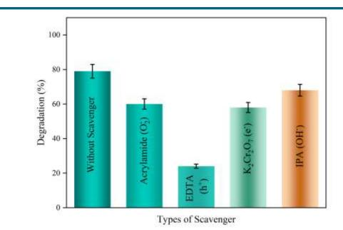
• The active species trapping experiment asserted that the degradation mechanism was controlled primarily by holes.
