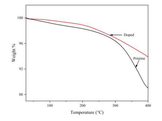
• Thermogravimetric analysis disseminated that the doping also improves the thermal stability of CsSnBr<sub>3</sub>; above 300°C, the difference in the stability becomes more perspicuous.
